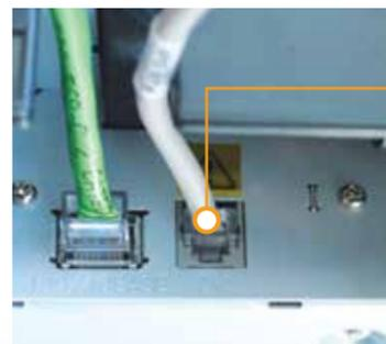
Connect the cash drawer cable (**GRAY CABLE**) underneath the cash drawer and into the "DK" port on the receipt printer.
