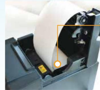
Remove the thermal paper from the wrapper and place into the printer with the roll facing out.
