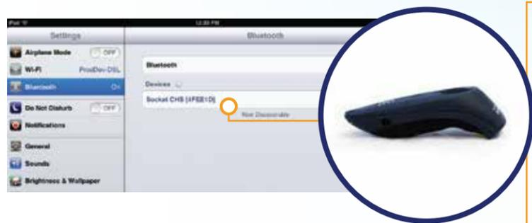
Turn on the scanner by pressing the smaller button on top of the scanner until it beeps twice, low to high.
